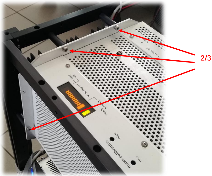
Figure 153: Mounting of the RF-Generator
